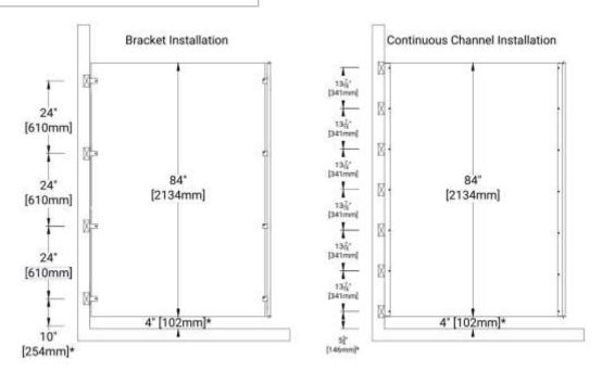
Note: Floor to ceiling pilasters to be installed with an AFF of 4 ½" (114mm).
