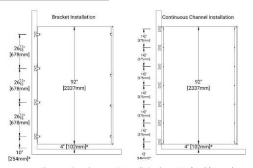
**Note:** Floor to ceiling pilasters to be installed with an AFF of 4 ½" (114mm).
