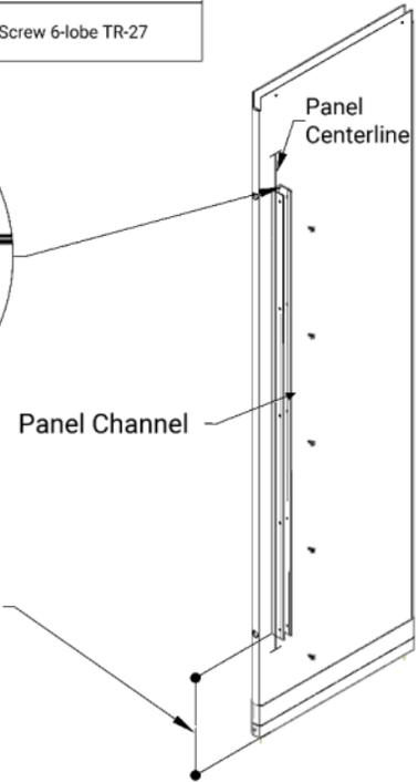
For a 102mm (4") above finished floor partition elevation, mount channel 111mm (4 3/8") above the finished floor.
