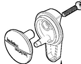
Install latch with thumb lever pointing downwards.
