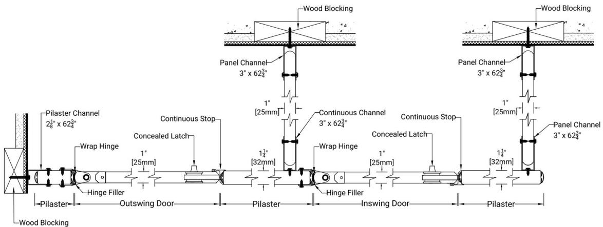
1" [25mm] x 1 5/8" [41mm] extruded anodized aluminum anti-grip headrail. Headrail sits 3/8" [3mm] above pilaster.
